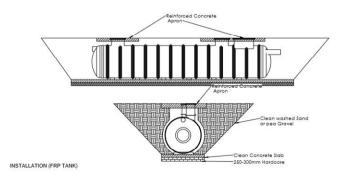
1. Excavate an area for positioning with suitable easy placing of the tank and filling as well as for consolidating concrete for backfilling.
