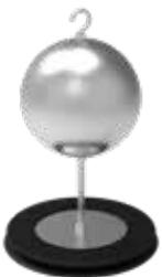
The automatic closure device is calibrated to float in water and sink in light hydrocarbon liquids. If the maximum oil spill capacity of the primary chamber reached, the device will shut off flow of liquid to the secondary chamber and therefore protecting the environment from a catastrophic event.
