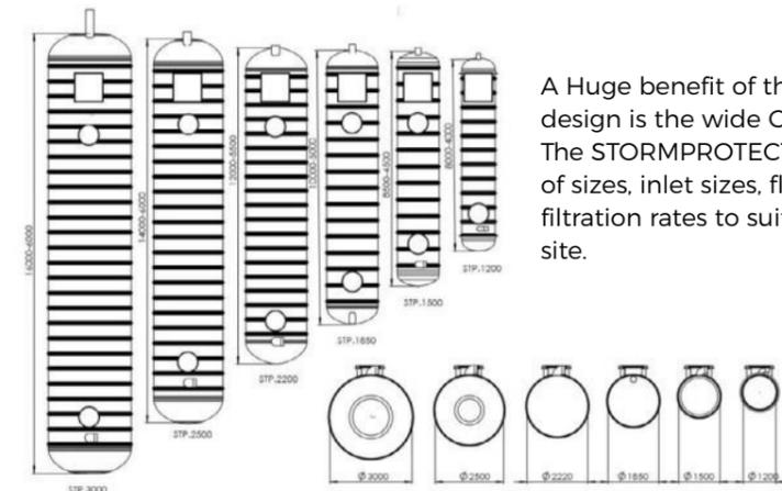
A Huge benefit of the STORMPROTECTOR design is the wide Configuration Range - The STORMPROTECTOR has a wide range of sizes, inlet sizes, flow rates and possible filtration rates to suit any demand of any site.
