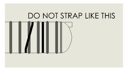
Straps must not be placed between the ribs or passed over from one side to the other as stress will be transferred to the weakest part of the tank wall. Unless the Protector system is used and position correctly to the instructions given the warrant will be nullified.
