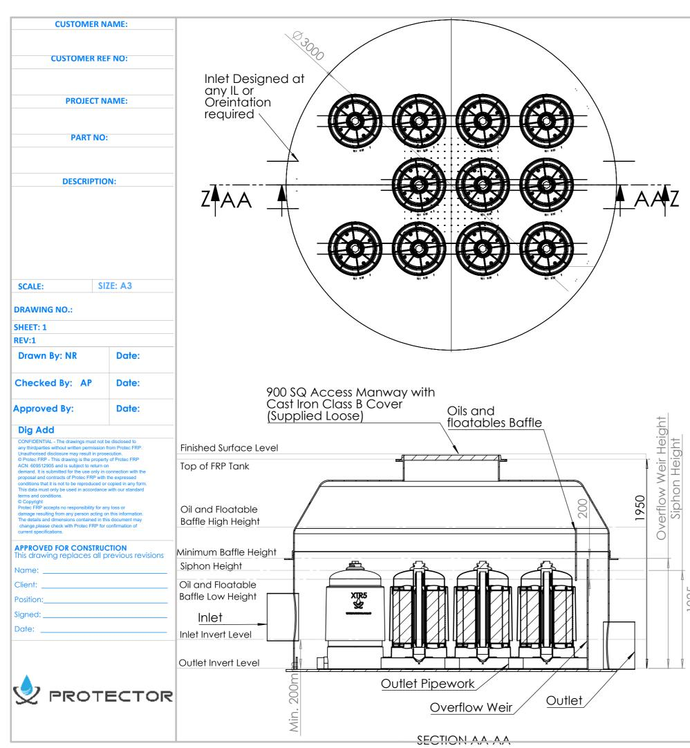
The Design Varies as per the number of filters per Water Quality Chamber. This drawing and details only apply to that of the current drawing
